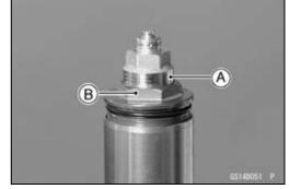
Avoiding the pins [A], set the front fork spring compressor set [B] on the washer [C].
