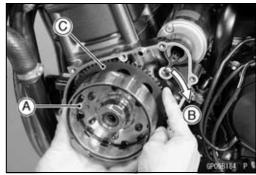
• Install the washer [A] so that the chamfer side [B] faces outward.
