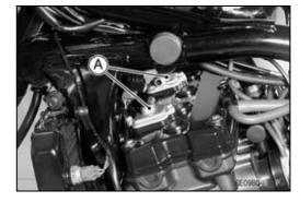
Remove the cylinder head cover bolts [A] and take off the cover.
