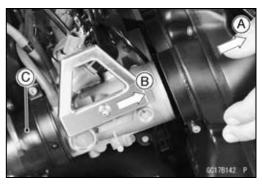
• Slide [A] the throttle body assy [B] left and remove it.
