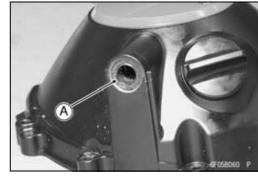
• Remove: Circlip [A]
