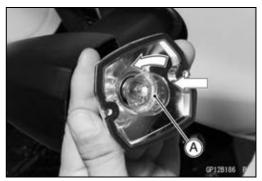
Insert the new bulb [A] by aligning its upper and lower pins
